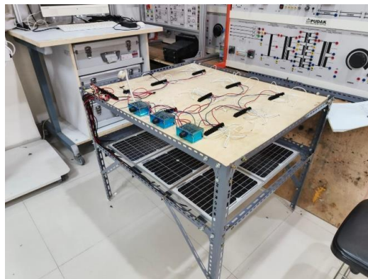
Figure 5. Solar Panel Simulator
