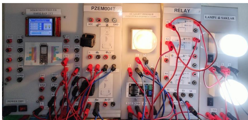
Figure 8. Results of Cable Assembly and Installation on the Trainer
