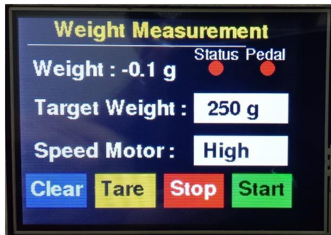
Figure 8. HMI display of 250 gram target weight measurement in High Speed
