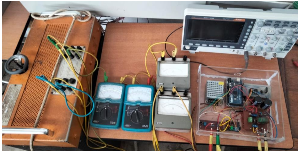
Figure 6. Hardware Boost Converter with Measuring Instrument
