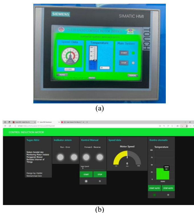
Figure 9. Automatic system operation with a temperature of 39°C (a) HMI and (b) PC
