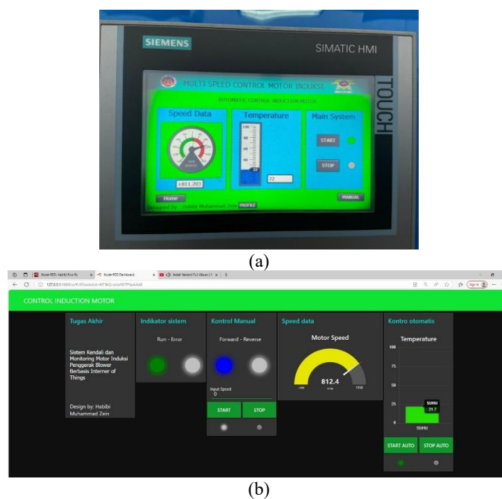
Figure 8. Automatic system operation with a temperature of 22°C (a) HMI and (b) PC
