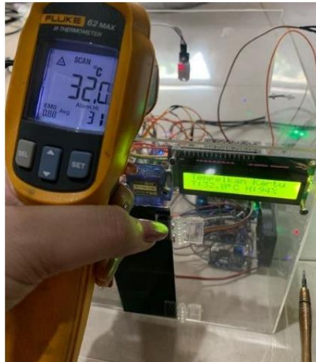
Figure 6. DHT22 Sensor Testing
