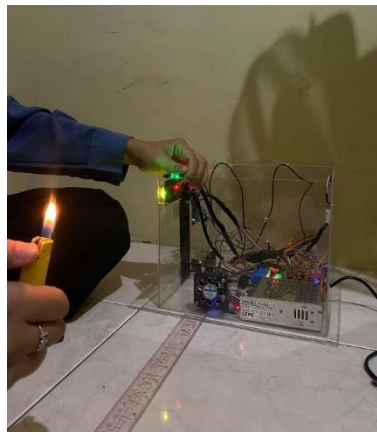
Figure 5. Flame sensor accuracy testing
