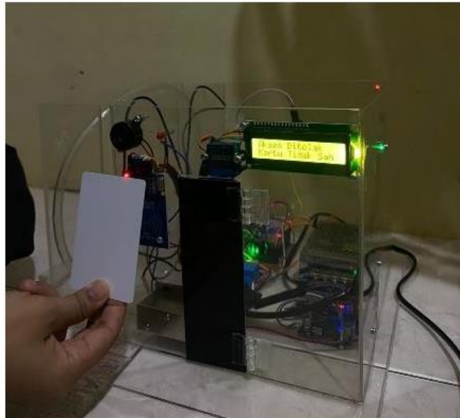
Figure 4. RFID Tag ID Reading Test
