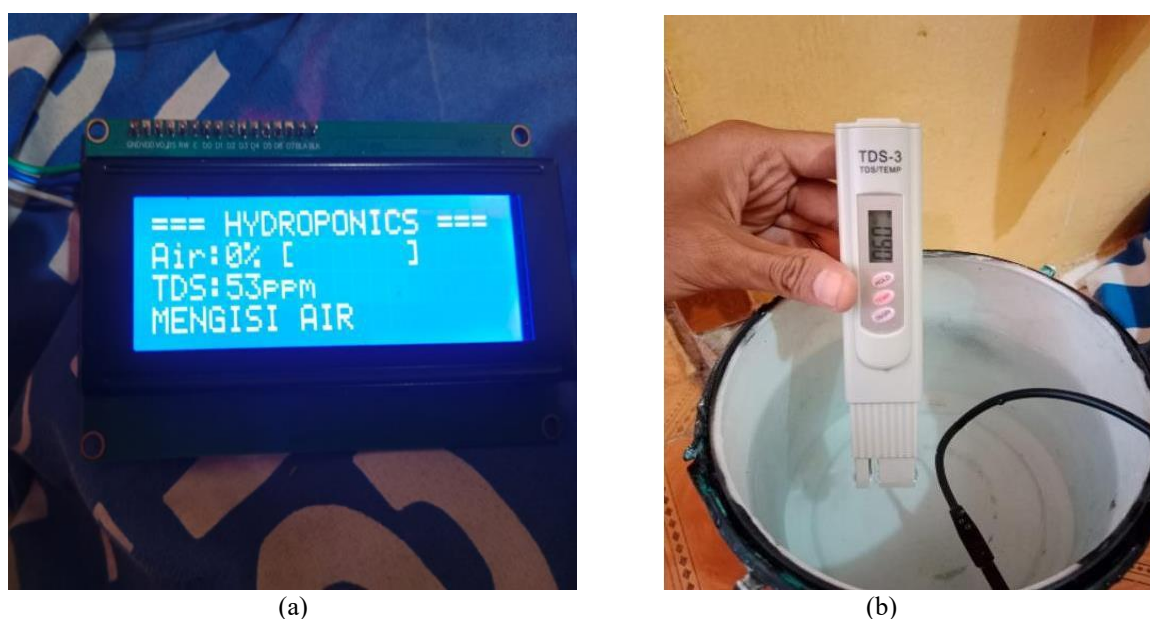
Figure 6. Experimental process. A) LCD display, b) Results using TDS Meter
