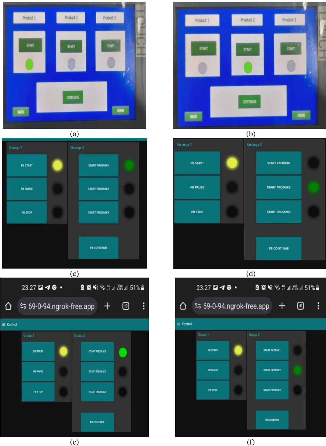
Figure 7. Display of HMI, PC server and smartphone, a) Activation of Product 1 button on HMI, b) Activation of Product 2 button on HMI, c) Activation of Product 1 button on PC server, d) Activation of Product 2 button on PC server, e) Activation of Product 1 button on smartphone, f) Activation of Product 2 button on smartphone
