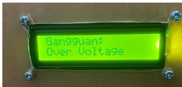
Figure 6. Overvoltage indicator on the LCD when there is an overvoltage disturbance
