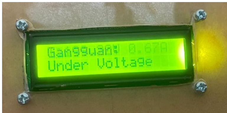
Figure 7. Undervoltage indicator on the LCD when there is an undervoltage disturbance
