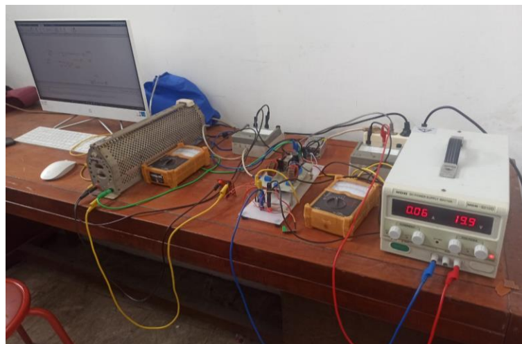
Figure 4. Experimental setup of quadratic boost converter
