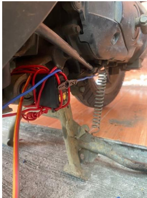
Figure 4. Mounting the Servo Motor to the Motorcycle
