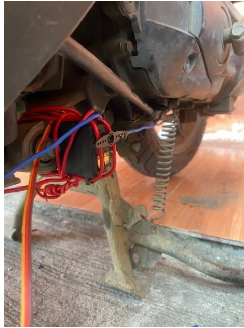
Figure 4. Mounting the Servo Motor to the Motorcycle
