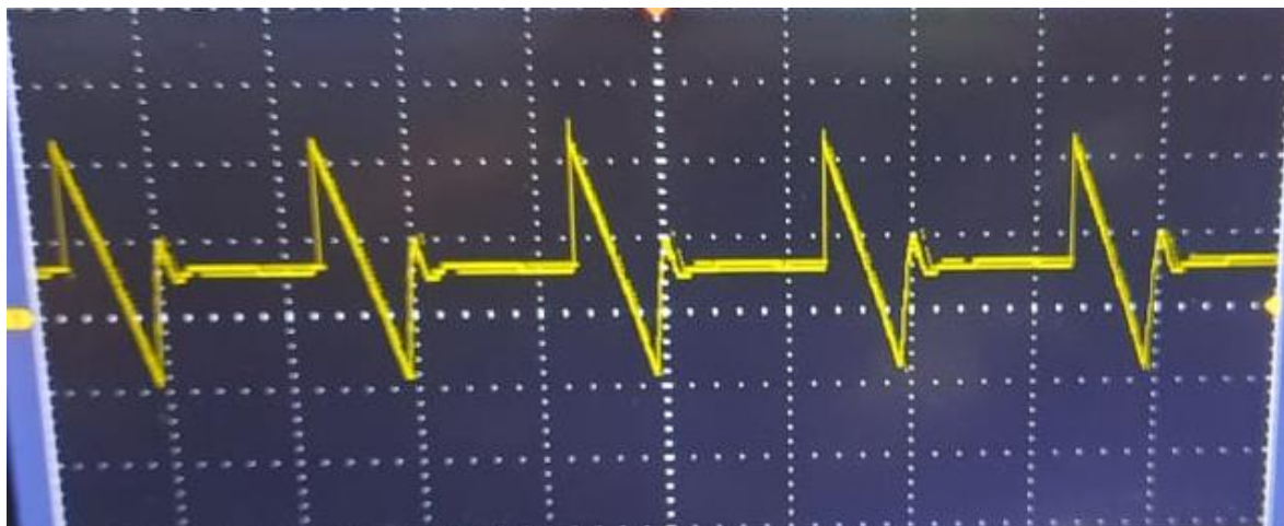
Figure 8. Rectifier output voltage graph
