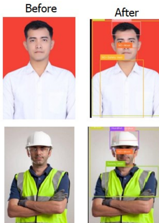
Figure 5. Results of Personal Protective Equipment (PPE) Usage Detector Test
