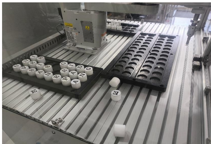
Figure 5. Workpiece Detaches From Vacuum Suction Cup
