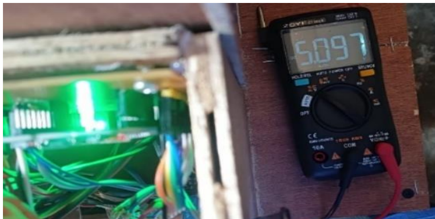
Figure 6. Stepdown module output voltage
