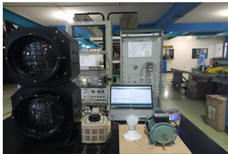
Figure 12. Testing of AC Motor Voltage and Current Conditions (Point Machine) at PT Len Railway Systems
