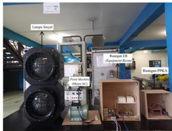
Figure 9. Results of making a prototype of an interlocking system
