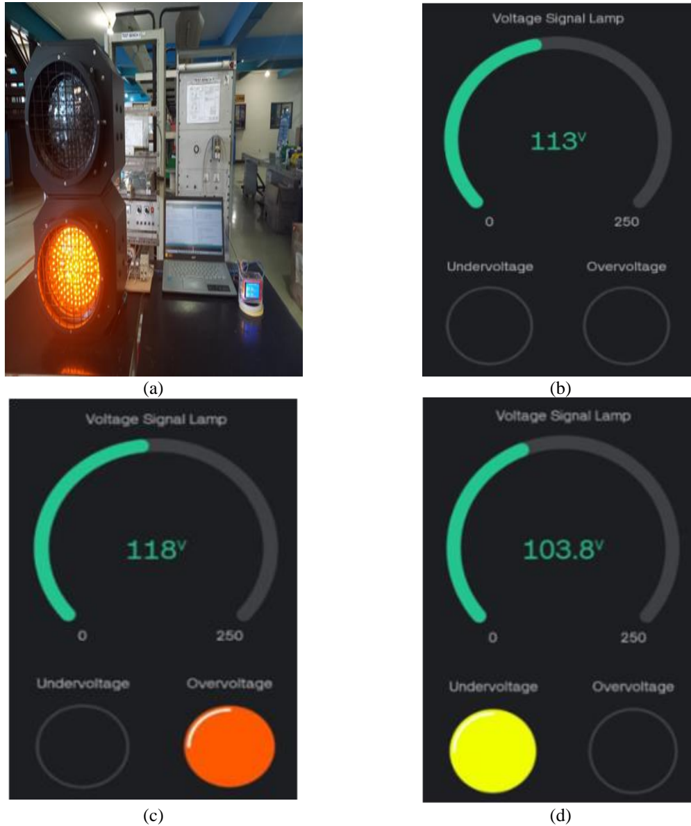
Figure 10. Lamp voltage testing, a) Testing process, b) first test, c) second test, d) third test
