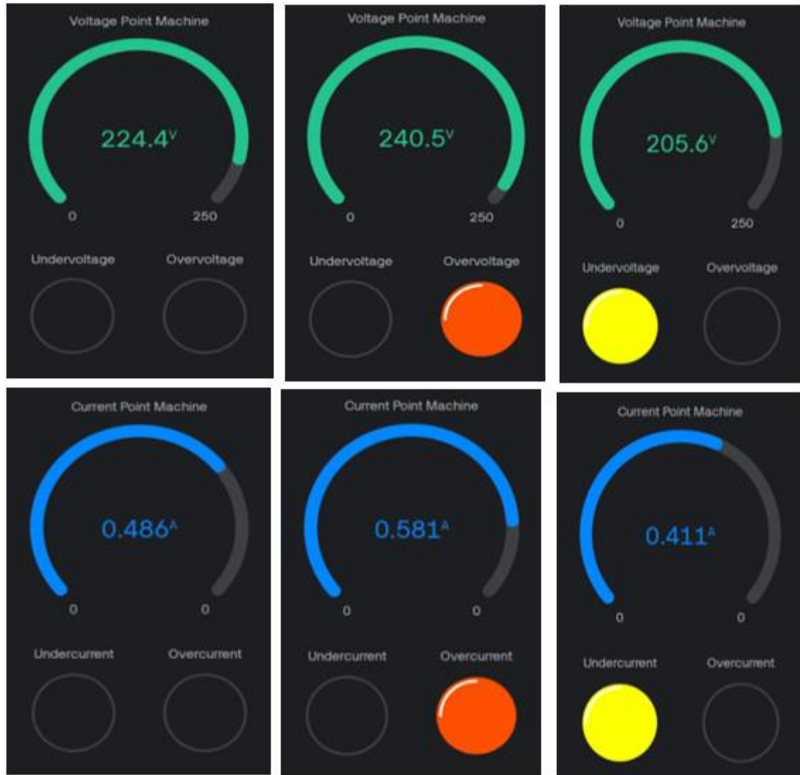
Figure 13. Monitoring display of AC motor current and voltage
