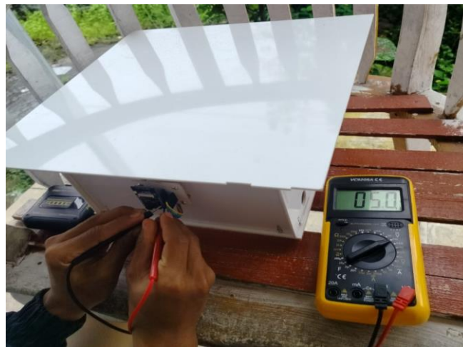
Figure 5. Measurement of ESP32-CAM input voltage
